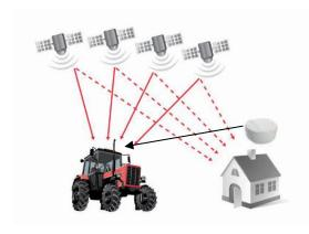
RTK base station: a fixed or mobile beacon present on the farm (or at a dealership) picks up satellites and calculates corrections RTK that it can transmit to the tractor via 2 different technologies: radio waves or GSM.
