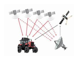
The signal transmitted by the GNSS satellites is picked up by a network of fixed reference EGNOS is spread over the European territory, which calculates correction and routes it to the receiver attached to the tractor via a geostationary satellite.
