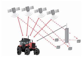
A network of reference stations quadrille territory (national or local). These reference stations are interconnected to a calculation that makes these corrections available via an Internet server. The tractor connects to the Internet via GSM, it transmits its position to the server, this one then puts personalized corrections to the service of the tractor.
